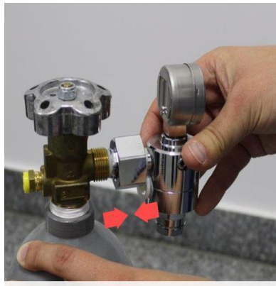
Attachment of the reducer to the cylinder
