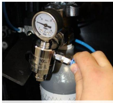
Pressure hose removal
