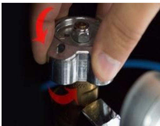
CO 2 cylinder opening direction
