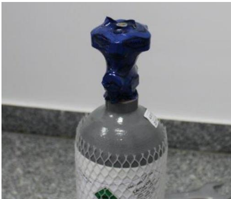
New cylinder - observe cylinder protection
