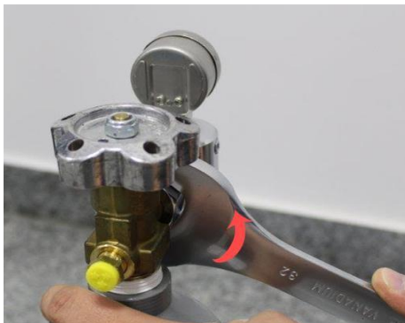
Reducer tightening (wrench upwards)
