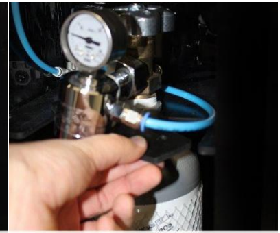
Cylinder fitting grip unlocking
