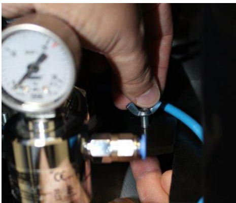
Tightening the grip fitting screw
