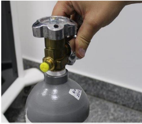
Unscrewing the pressure reducer
