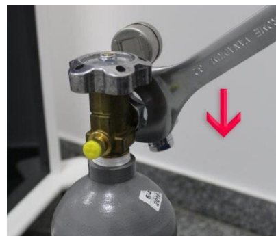
Loosening the reducer to the left (wrench no. 32)
