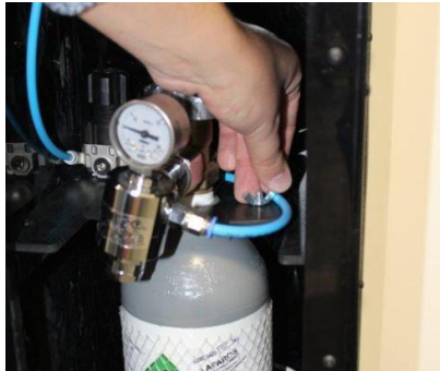
Grip fitting screw loosening
