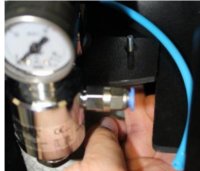
Attachment of the cylinder fitting grip
