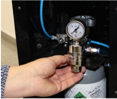
Attachment of the cylinder fitting grip
