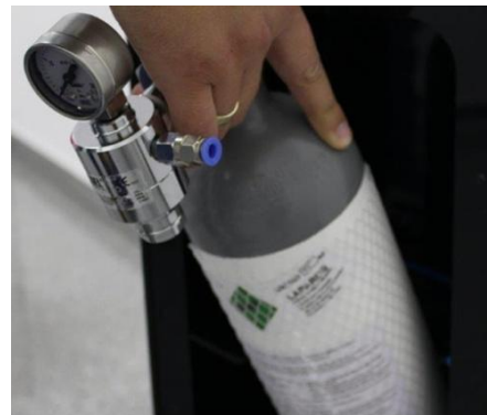
Inserting the cylinder in the device
