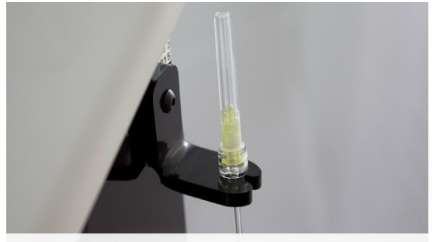
Properly attached needle on the grip
